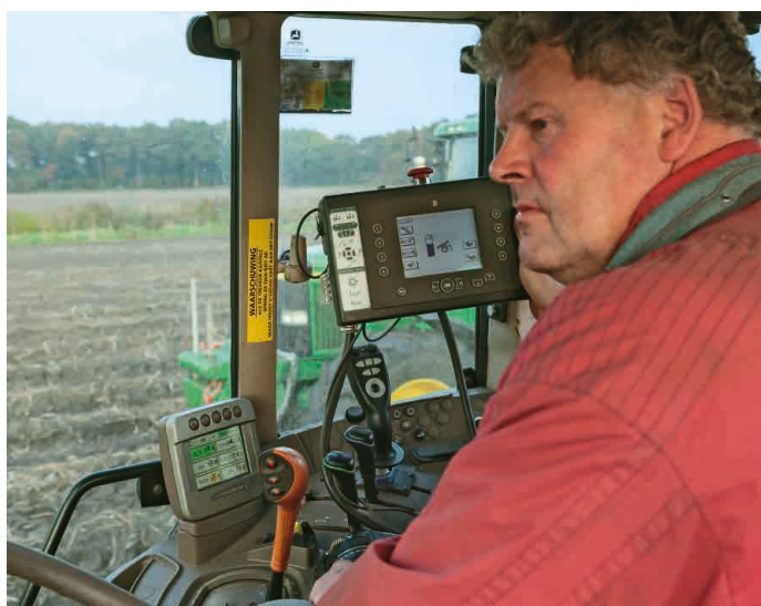
■ CAN-bus operation with joystick and control box
